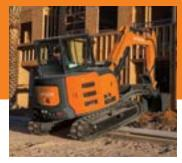
Choose the tracks that are best for the way you work. The rubber tracks traverse virtually any terrain, including paved surfaces. Also available are steel tracks and steel tracks with rubber pads. The optional rubber grousers combine workanywhere flexibility with steel-track serviceability.
