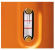
■ Hydraulic fluid sight gauge and see-through coolant reservoir let you quickly check levels at a glance.
