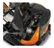
Operator station tilts forward 50 degrees, simplifying access to the swing motor, hydraulic control valve, engine starter motor and alternator.
