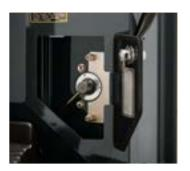
■ Go from backhoe- to excavatorstyle controls with just a twist of your wrist. Control-pattern selector valve is conveniently located in a compartment beneath the seat.
