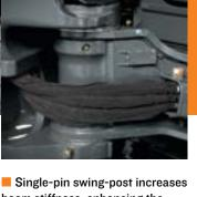
■ Single-pin swing-post increases boom stiffness, enhancing the structural integrity of the digging components. Wear-resistant hoses are routed for protection and Cordura®-wrapped where exposed.
