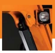
Heavy-duty shields deflect material and impacts, protecting the boom/blade cylinders and drive motors.
