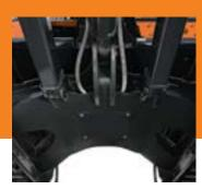
■ Heavy-duty X-frame provides a solid, stable platform that resists material and dirt build-up.
