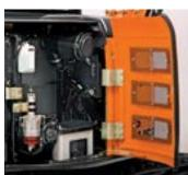
■ Hinged door provides wideopen access to the side-by-side oil cooler and radiator for easier core cleanout.
