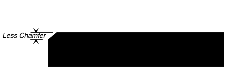
Fig. 6-20: Pad Worn, But Still OK
